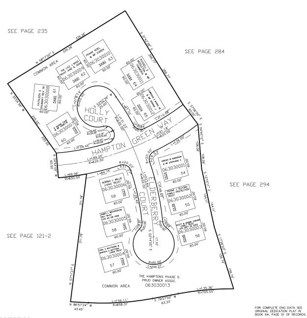
10' UTILITY & DRAINAGE EASEMENTS EACH SIDE DF PROPERTY LINES AS INDICATED BY DASHED LINES EXCEPT AS OTHERWISE SHOWN.
